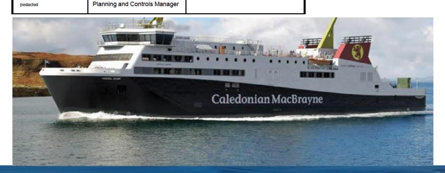
100m LNG Dual-fuelled Ro-Ro Passenger Ferry
