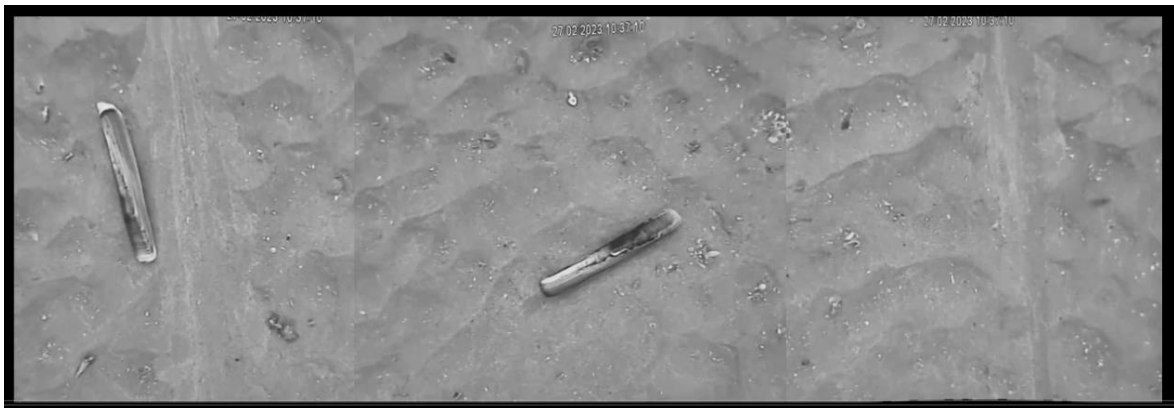
Figure 10: Example of image quality from stitching the three MacArtney Luxus camera feeds to generate a composite image equivalent to 1.5 m width on the seabed (tow 42, 27 February 2023 recorded in 15 m water depth). The trail marks left in the sand by the electrodes are also visible.
