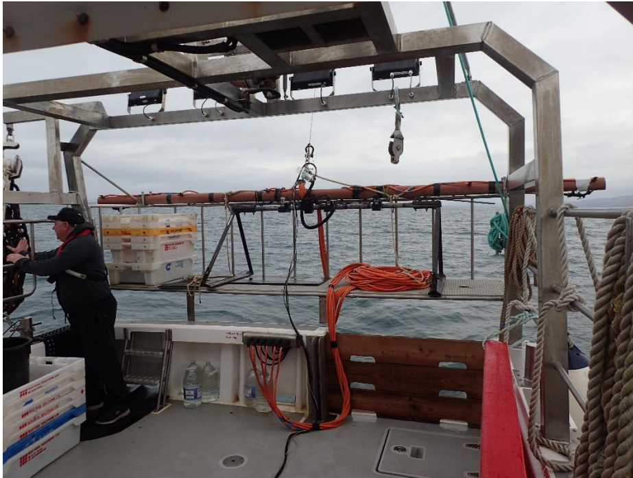
Figure 5: Aft deck of fishing vessel 'Skye' showing the raised platform with electrical cables, electrode spreader bar and the towed video rig stowed during passage.
