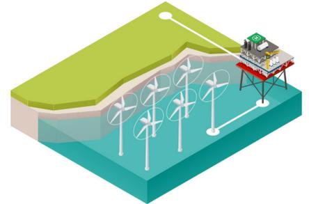
**Scenario 3** – Commercial scale offshore wind farm coupled with offshore hydrogen production.
