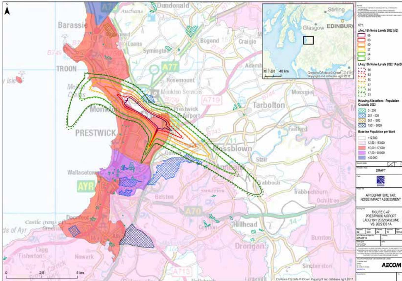
Figure C.50 Prestwick Airport Baseline 2022 v Scenario 1c L<sub>night</sub> dB Noise Contours
