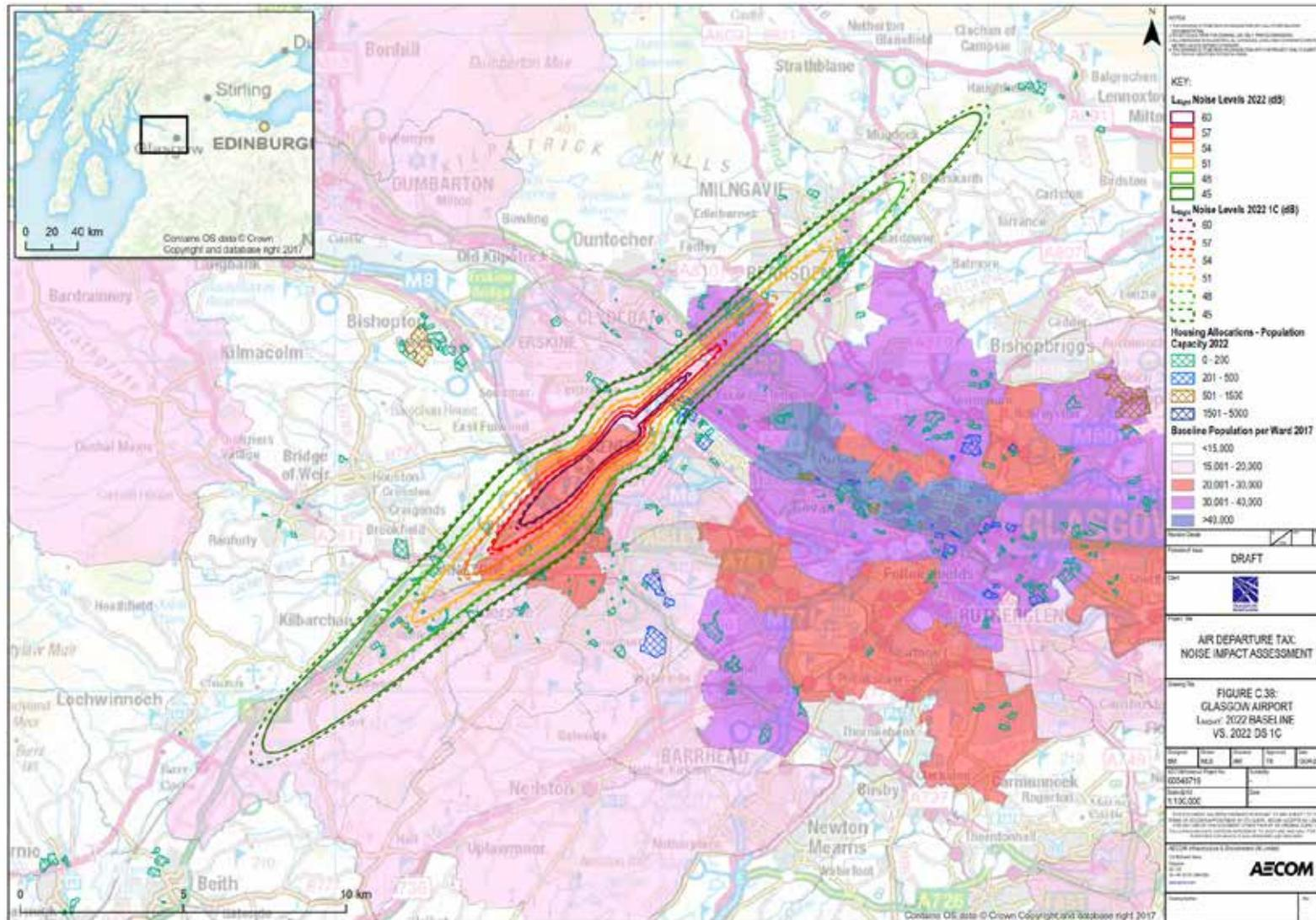
Figure C.39 Glasgow Airport Baseline 2022 v Scenario 2a  $L_{Aeq,16h}$  dB Noise Contours
