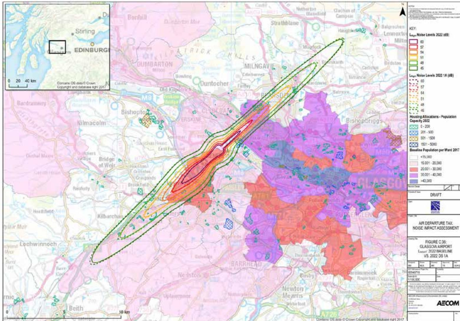
Figure C.37 Glasgow Airport Baseline 2022 v Scenario 1c  $L_{Aeq,16h}$  dB Noise Contours
