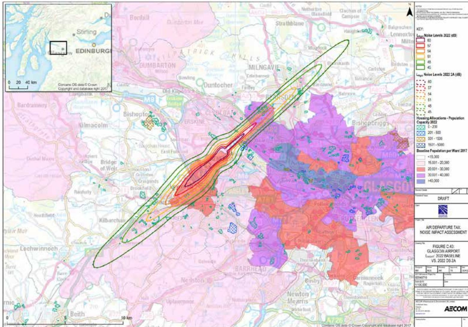
Figure C.41 Glasgow Airport Baseline 2022 v Scenario 2c  $L_{Aeq,16h}$  dB Noise Contours
