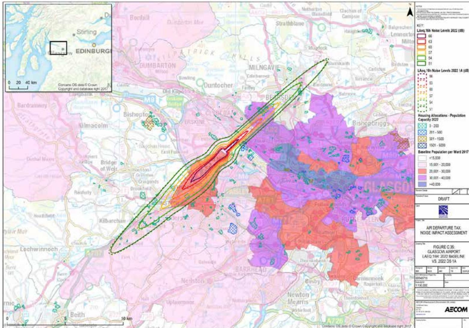
Figure C.36 Glasgow Airport Baseline 2022 v Scenario 1a L<sub>night</sub> dB Noise Contours
