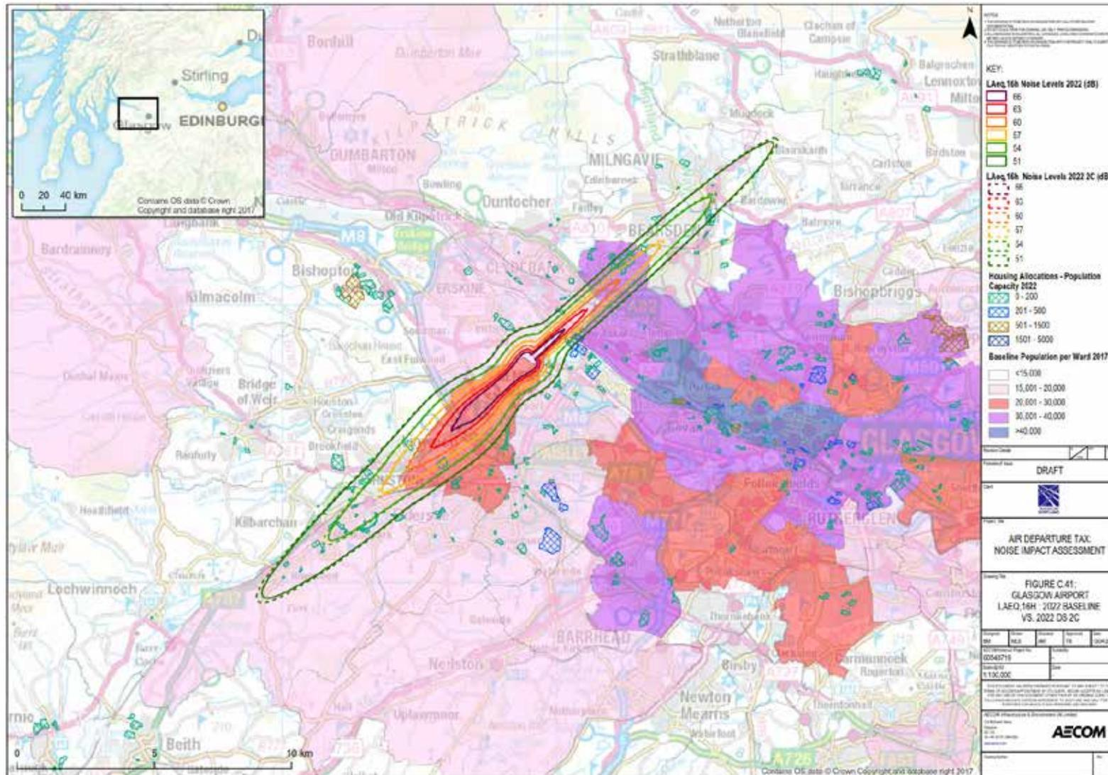
Figure C.43 Glasgow Airport Baseline 2022 v Scenario 3a  $L_{Aeq,16h}$  dB Noise Contours
