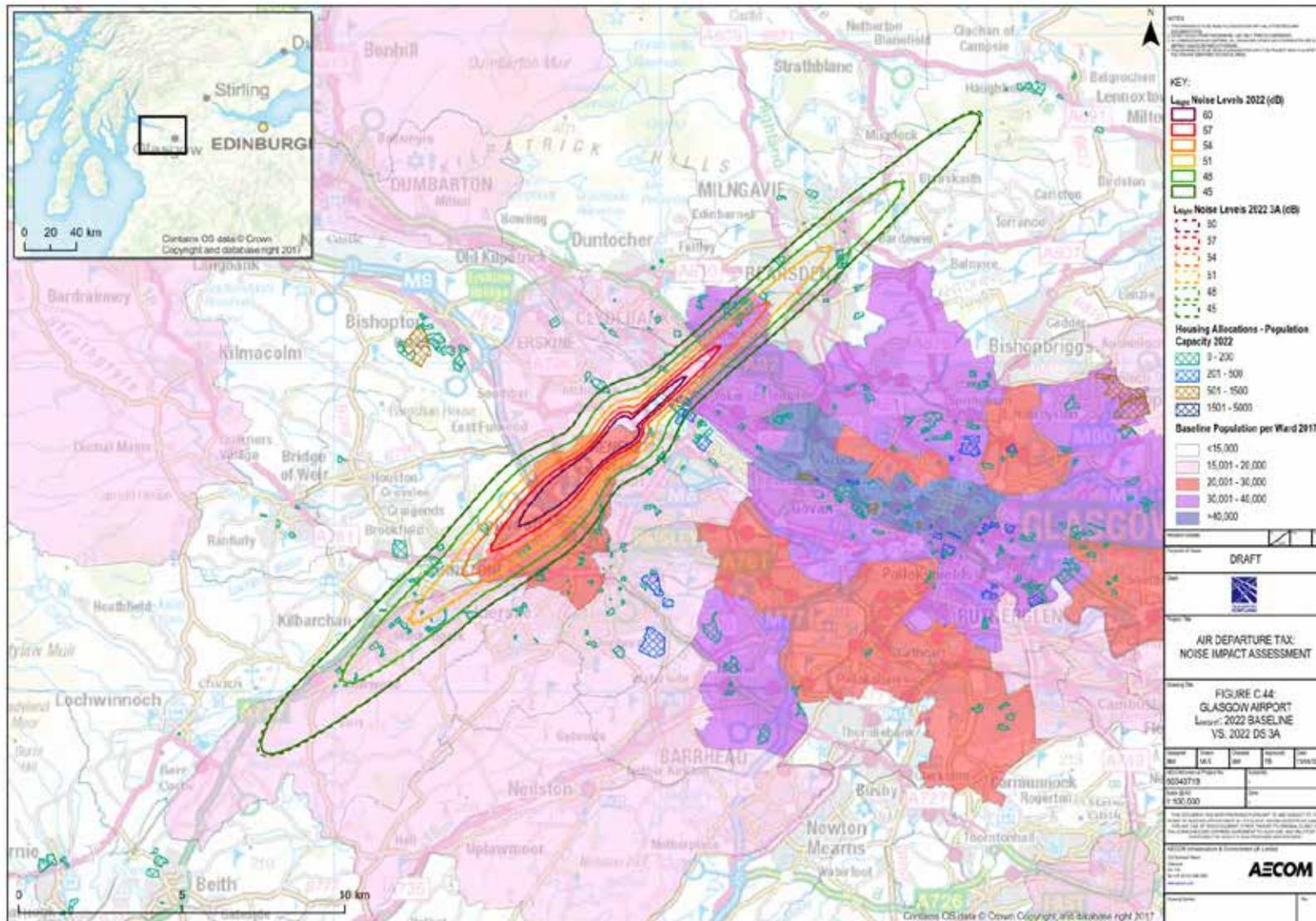
Figure C.45 Glasgow Airport Baseline 2022 v Scenario 3c  $L_{Aeq,16h}$  dB Noise Contours
