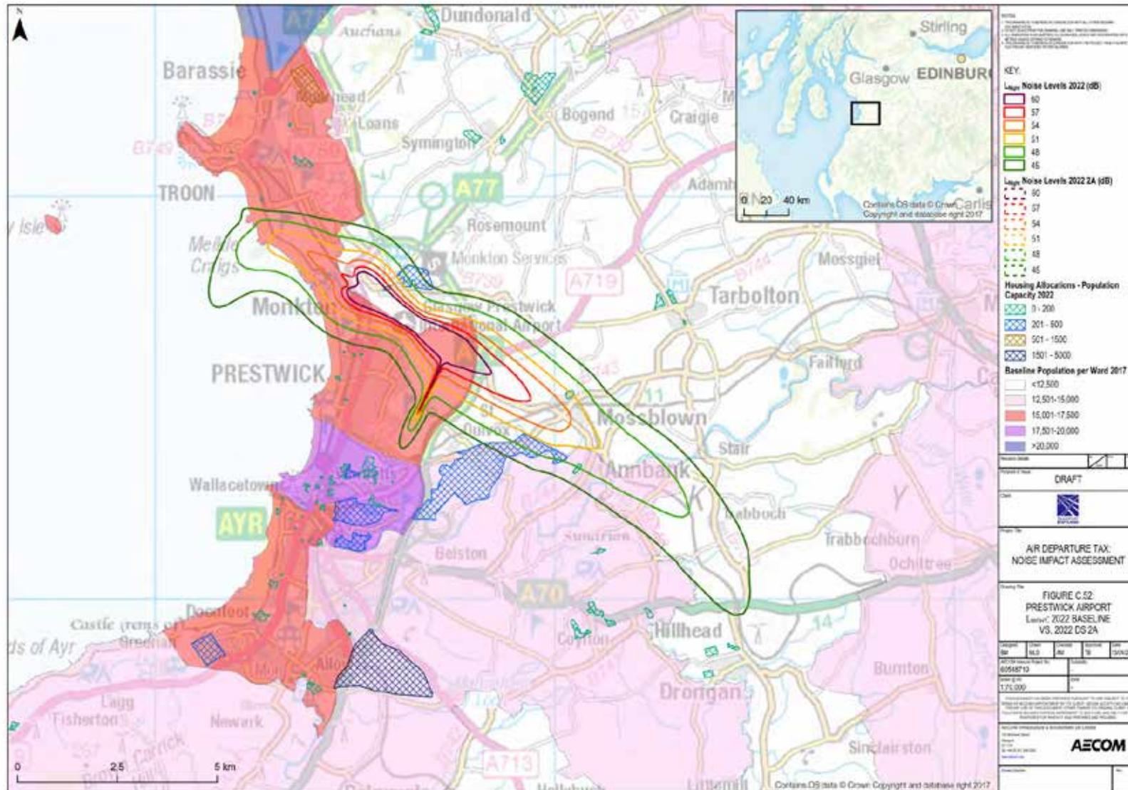
Figure C.55 Prestwick Airport Baseline 2022 v Scenario 3a  $L_{Aeq,16h}$  dB Noise Contours
