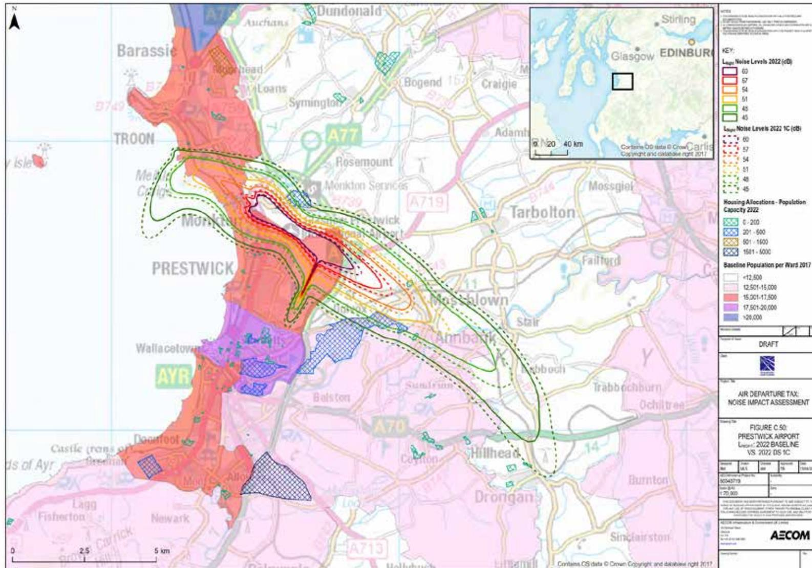
Figure C.51 Prestwick Airport Baseline 2022 v Scenario 2a  $L_{Aeq,16h}$  dB Noise Contours
