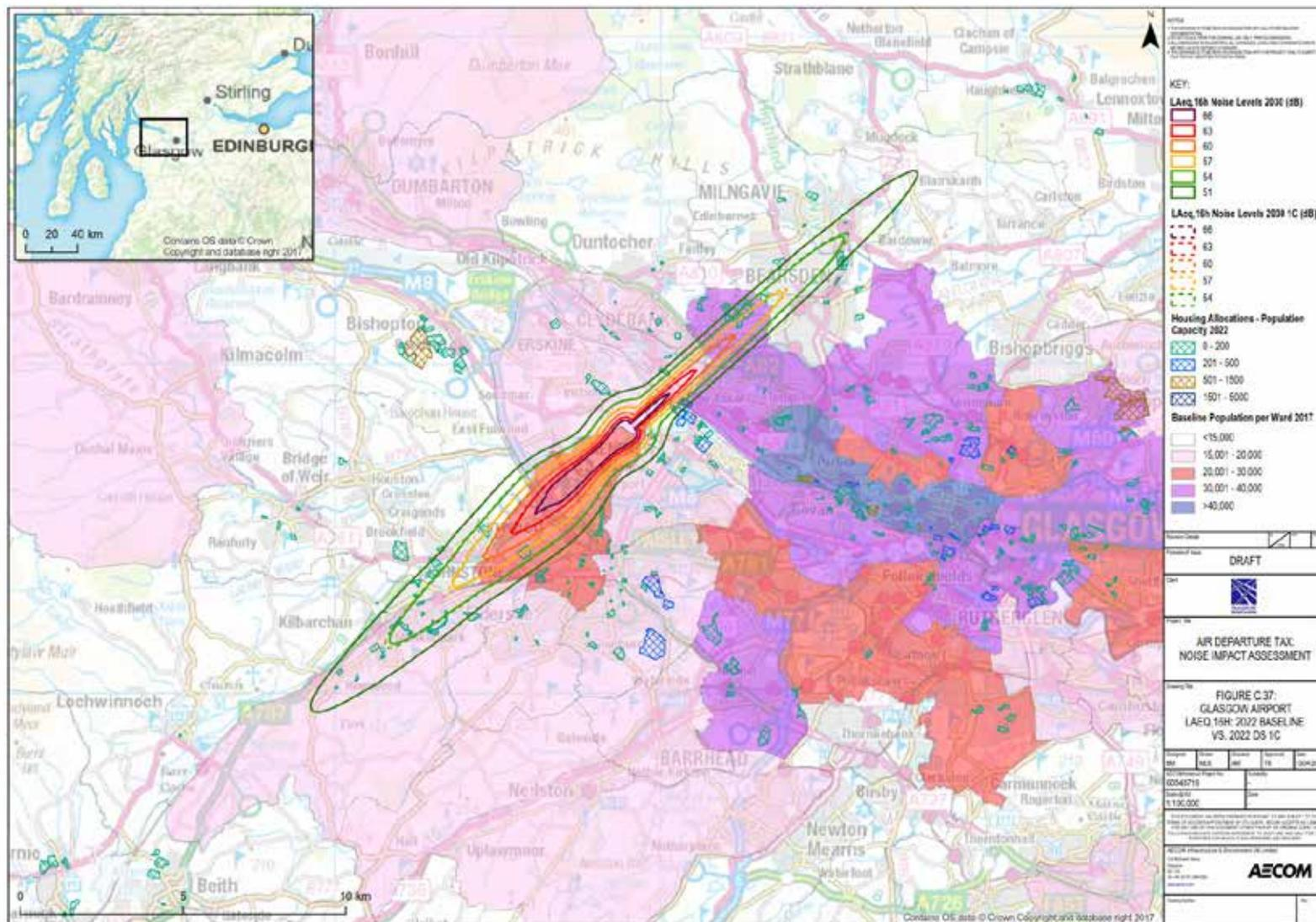
Figure C.38 Glasgow Airport Baseline 2022 v Scenario 1c L<sub>night</sub> dB Noise Contours
