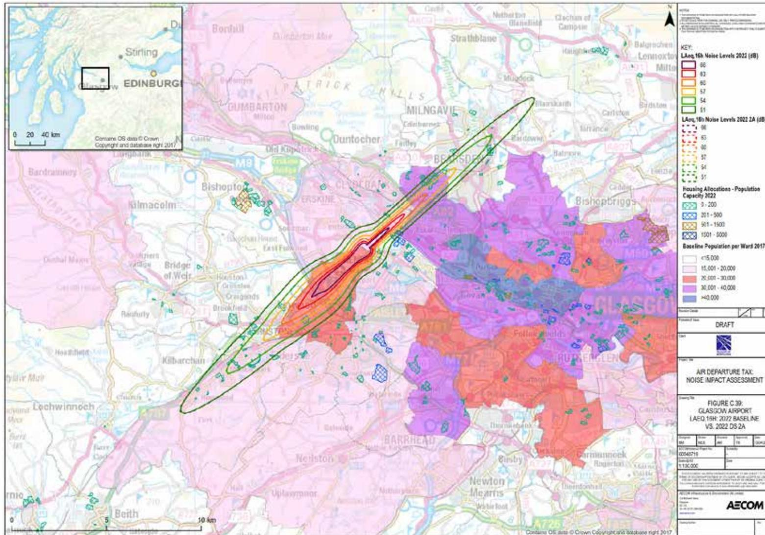
Figure C.40 Glasgow Airport Baseline 2022 v Scenario 2a L<sub>night</sub> dB Noise Contours
