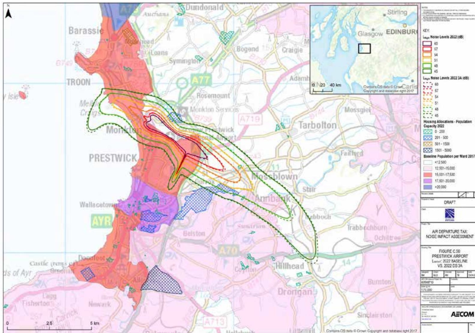
Figure C.58 Prestwick Airport Baseline 2022 v Scenario 3c L<sub>night</sub> dB Noise Contours
