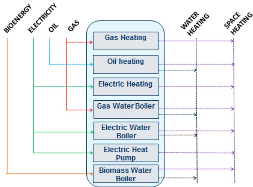
Figure 4: Based on “Using the TIMES model in developing energy policy, 2017”<sup>2</sup>
