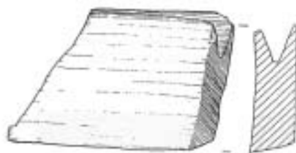
Example of a fragment of oak cladding from Edinburgh
