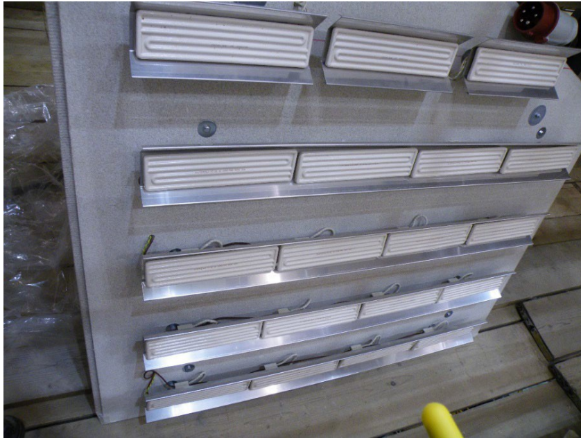
Typical heating array panel
