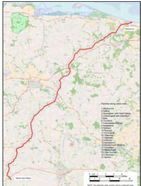
Figure 4: Showing the route of the cable from Weybourne to the substation at Necton from the Dudgeon Offshore Wind Farm;
