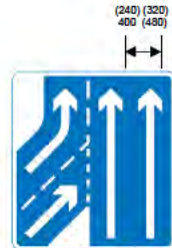
873 Additional traffic lane joining from left ahead. Traffic on main carriageway has priority over joining traffic from the right hand lane of the slip road.
