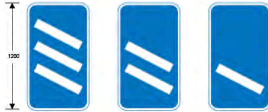
823,824,825 Distance in hundreds of yards to a roundabout or the next point at which traffic may leave a route
