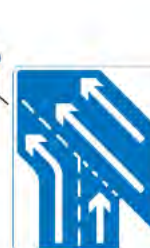
874 Additional traffic lanes joining from the right ahead. Traffic in the right hand lane joins the main carriageway. Traffic on the main carriageway has priority over joining traffic.
