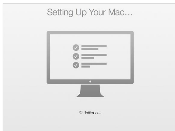
Figure 6.3 - macOS Setup Wizard automatically applying configuration, policy and profiles as defined in DEP
