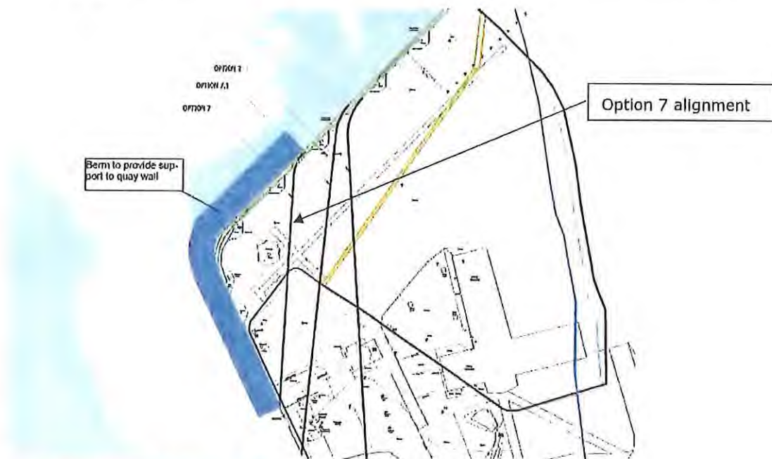
Figure 14 Construction Method B - Plan
