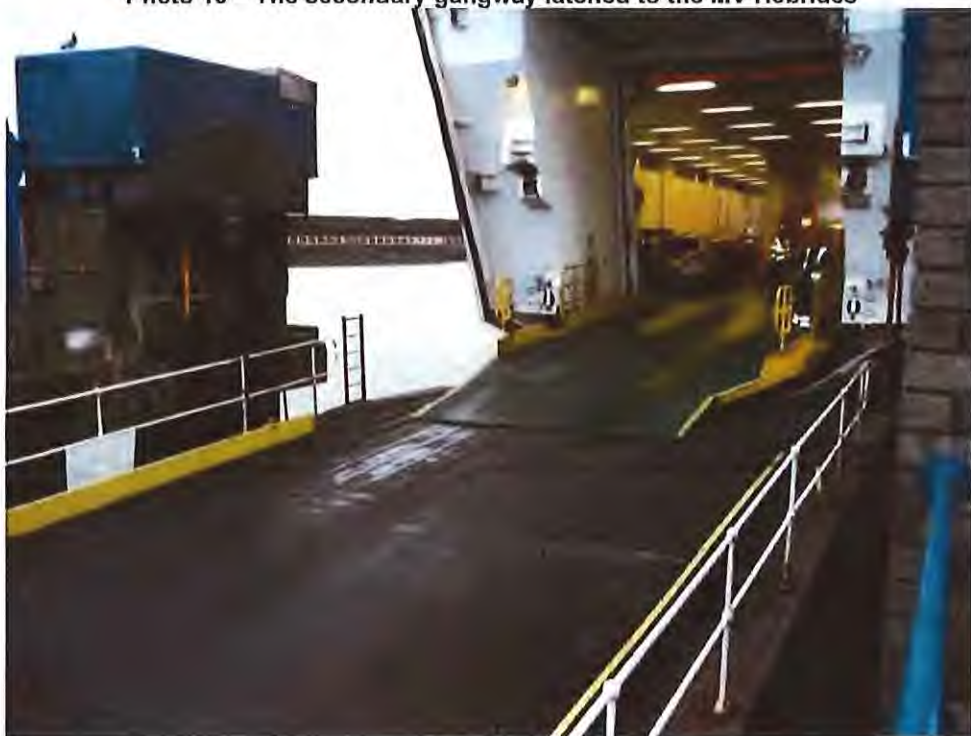
Photo 10 – The secondary gangway latched to the MV Hebrides
