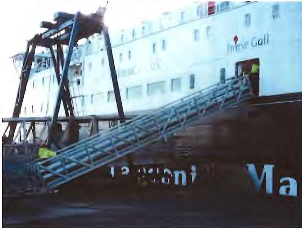
Photo 10 – The secondary gangway latched to the MV Hebrides
