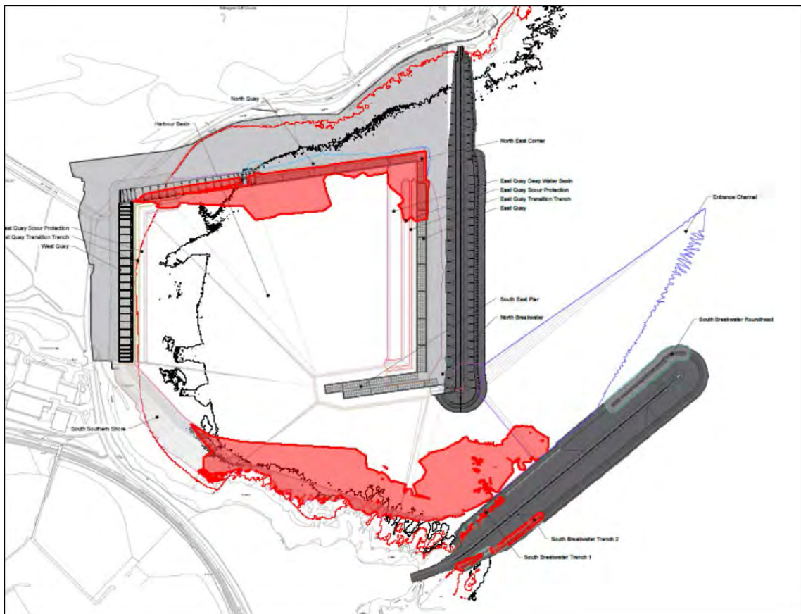
Figure 3.1 - Rock Blasting Zones – North and South (Final Definitive Blasting Areas)
