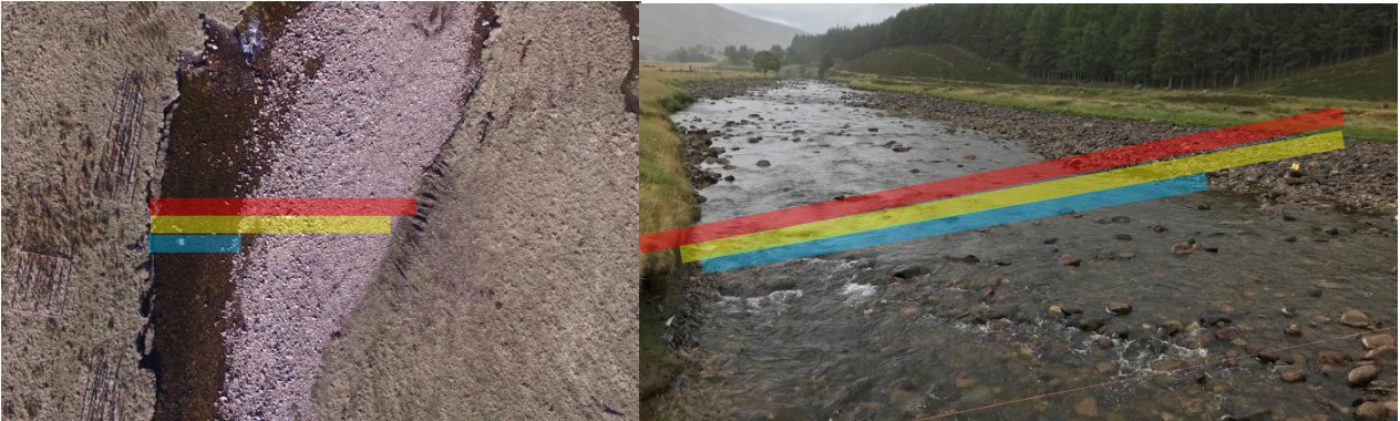
Figure A1.1 Width measurements where blue denotes wetted width, yellow denotes bed width (active channel) and red denotes bank full width
