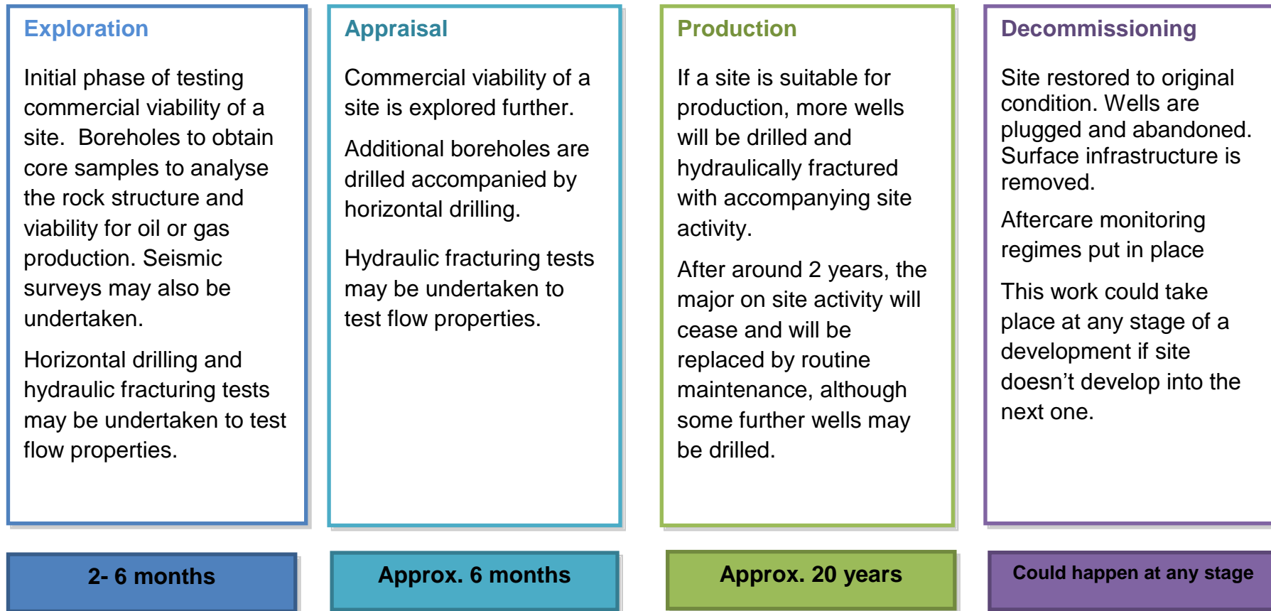
Figure 2: Stages of a typical UOG development. Timeframes are indicative and do not include the time taken to secure relevant consents.
