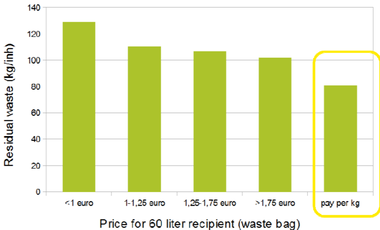
Figure 4: Residual waste per capita per year in Flanders between a weight-based system and cost per bag in a volume-based system. 154
