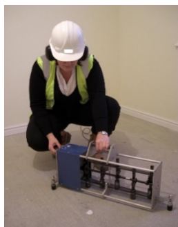
Figure 4 Impact sound test being carried out
