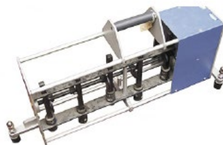
Figure 5 Typical tapping machines for impact sound insulation tests
