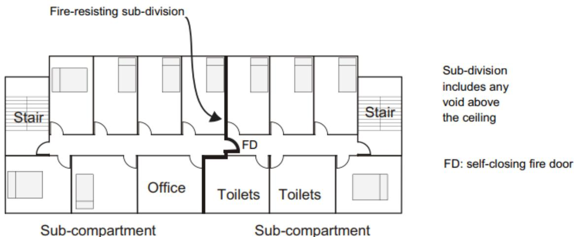
**Figure 3** Plan layout of an upper floor of a care home which is sub-divided into two sub-compartments
