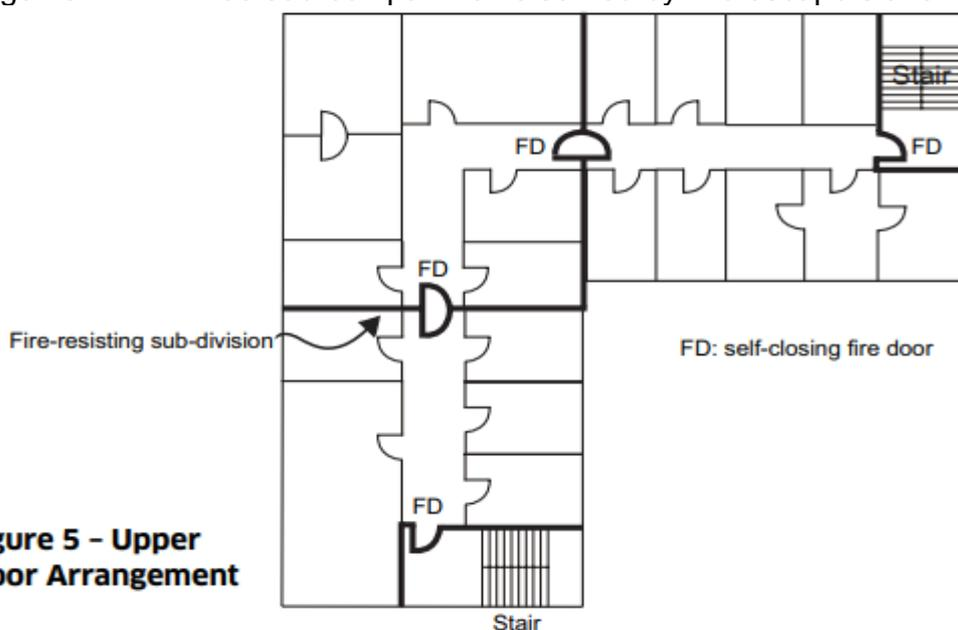
202. A room with an occupant capacity of more than 60 should have at least two exits. The direction of travel of alternative escape routes from any point within the room should:
