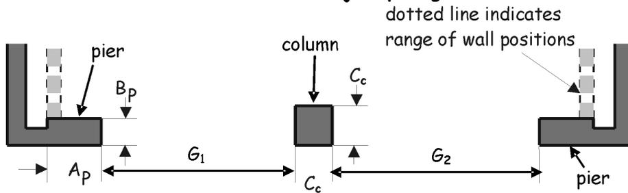
**1.D.42 Horizontal lateral restraint at roof level**
