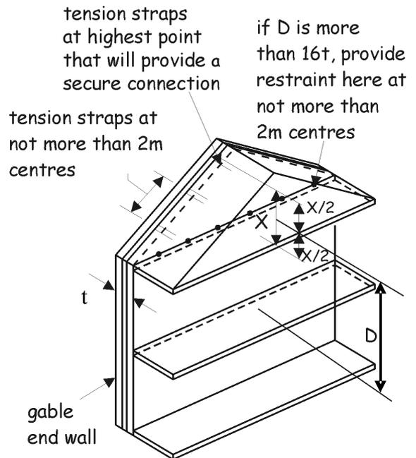
The wall thickness,  $t$  = sum of the thicknesses of the leaves + 10 mm.
