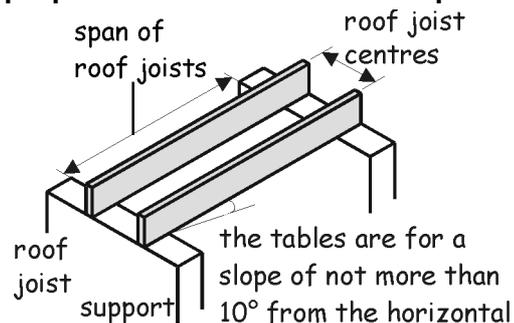
**Permissible clear spans, in metres, of joists for flat roofs with access only for maintenance or repair purposes**
