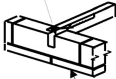
internal leaf of external cavity wall with lateral restraint
