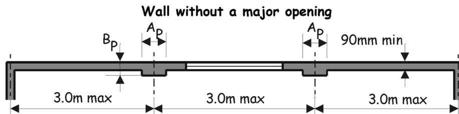
Walls which contain 1 or 2 major openings should, in addition, have piers oriented as shown in the diagrams above, opposite and below. Where ties are used to connect piers to walls they should be flat, 20 mm x 3 mm in cross
