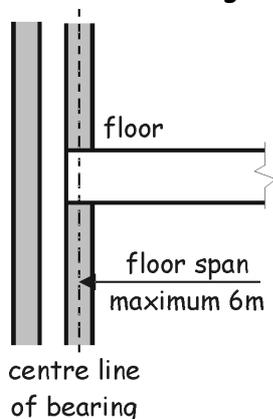
Floor member bearing on joist hanger
