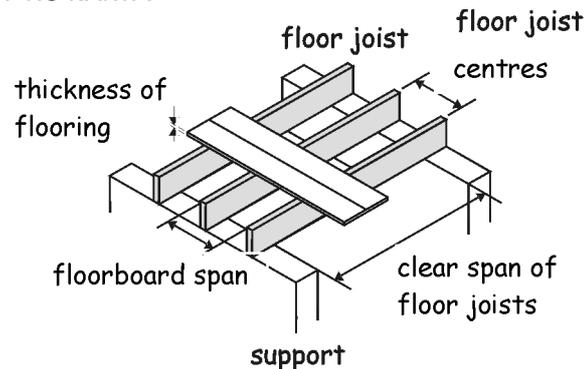
**Permissible clear spans, in metres, of joists supporting floors with no partitions
