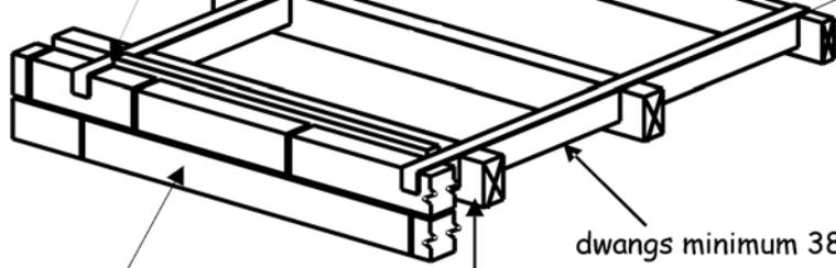
joist blocked to wall
