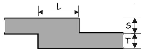
$$L = \text{greater of } 2 \times S, T, \text{ or } 300 \text{ mm}$$
