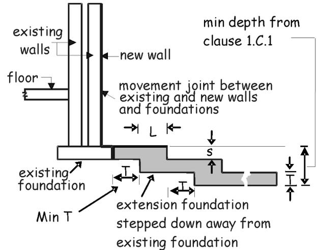
To minimise the risk of differential settlement occurring between the extension and the existing structure, the following should be considered:
