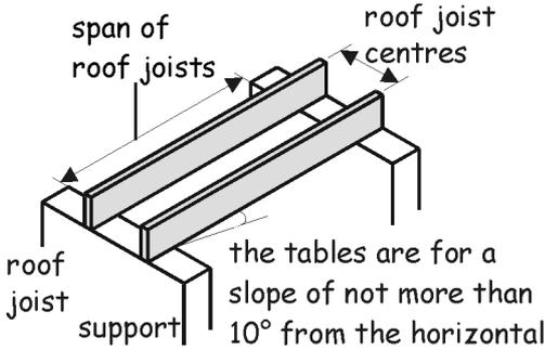
**Permissible clear spans, in metres, of joists for flat roofs with access not limited to maintenance or repair purposes**
