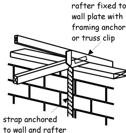
**Vertical strapping at eaves of flat roof**
