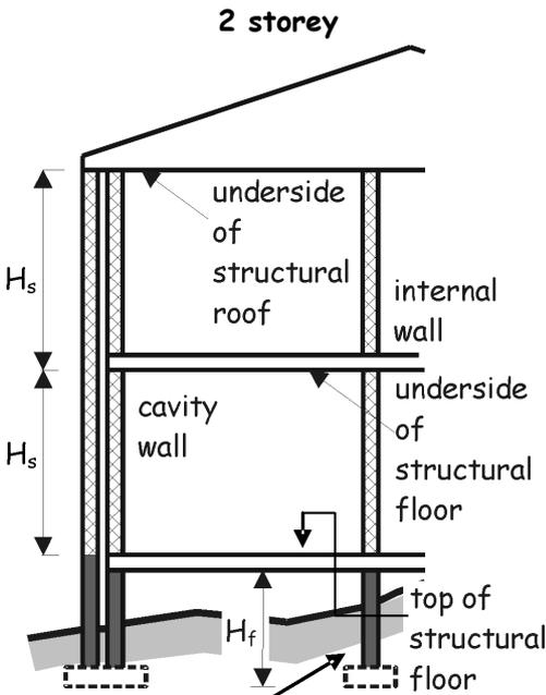
this wall to be at least 140 mm thick in blockwork or 215 mm thick in brickwork below ground floor level if height  $H_f$  is more than 1m.
