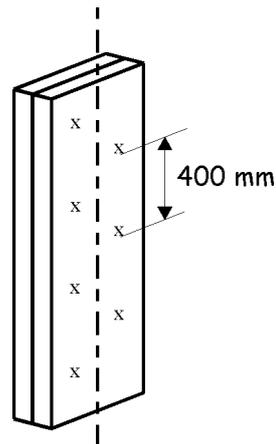
Lintels should be secured to each other with 3.1 mm x 75 mm galvanised screws or 3.1 mm x 75 mm galvanised ringshank nails at 300 mm centres, staggered mid distance between edge and centreline, with no screw closer than 60 mm to end of lintel.
