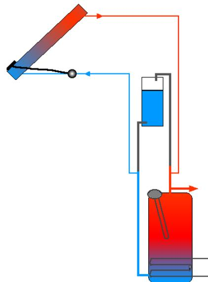
**Figure 2: Example of a direct pumped solar water heating system (with PV-powered pump)**
