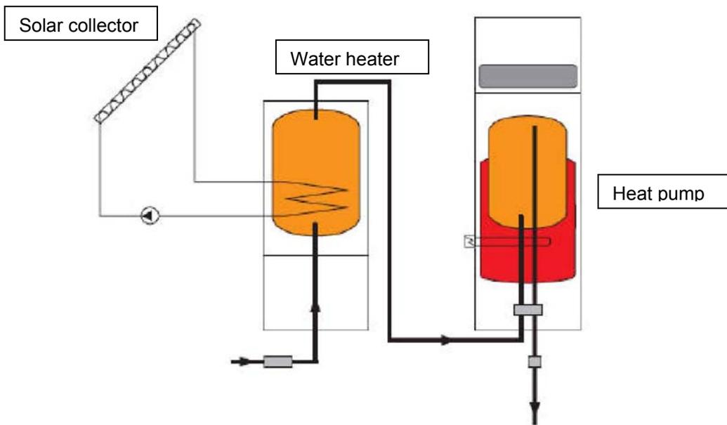
**Figure 9: Solar water heating supplementing heating by a ground source heat pump**
