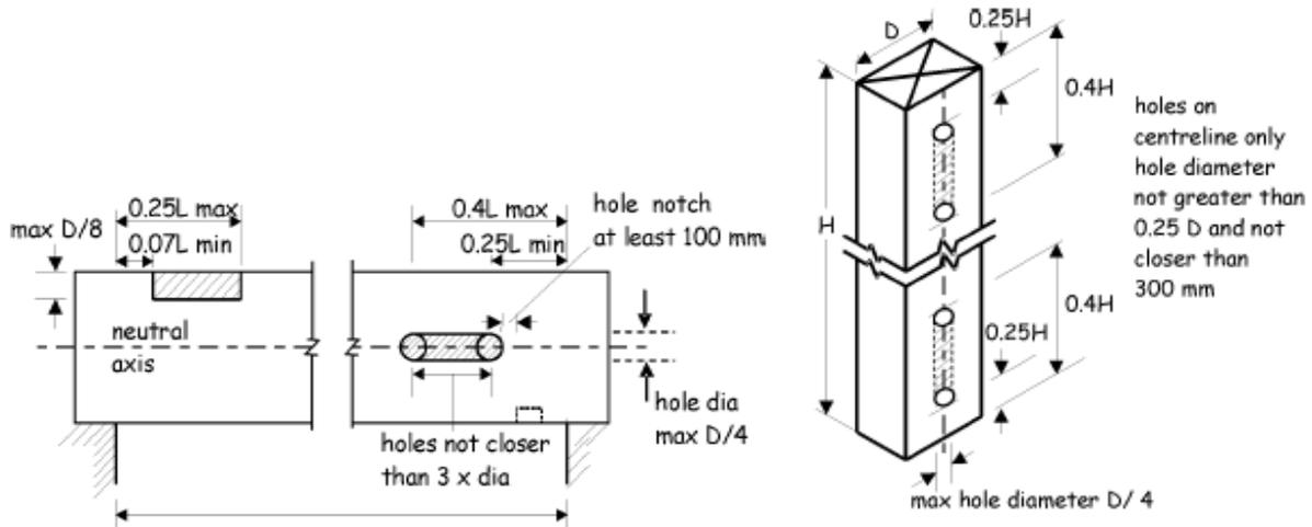
**Figure 11: Notches and hole locations in timber floor joists and studs**
