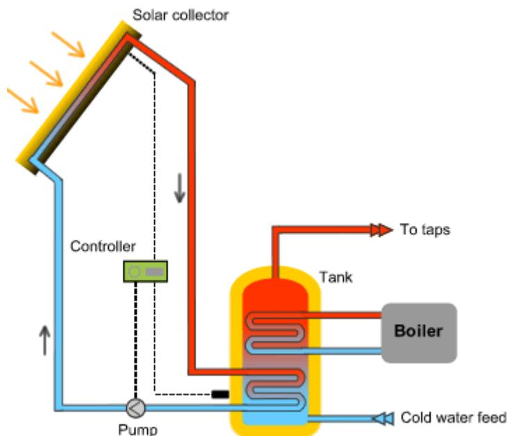
**Figure 1: Example of an indirect pumped solar water heating system, with twin-coil storage**
