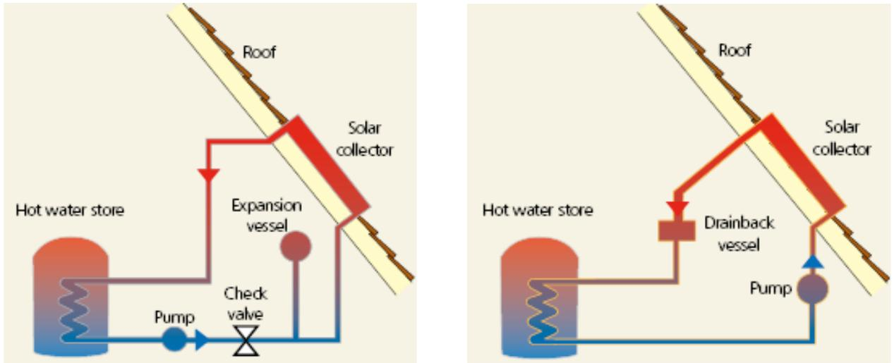
**Figure 3: Schematic of a) typical fully filled indirect system b) typical drainback indirect system**
