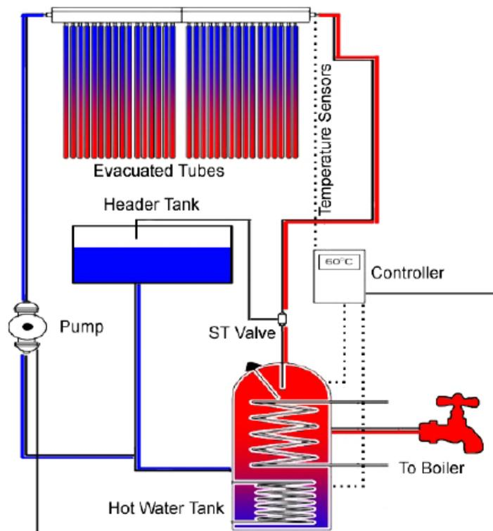
**Figure 4: Example of an open vented system using evacuated tubes**
