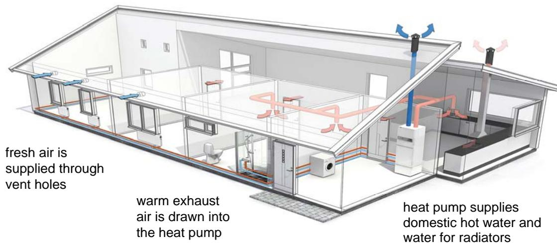
**Figure 7: Whole house ventilation system with heat pump**
