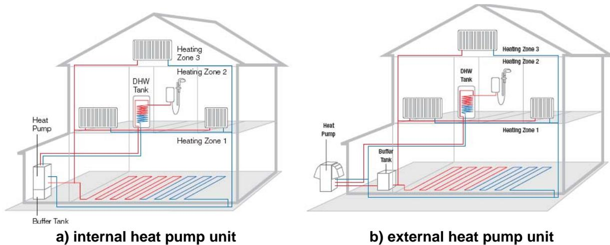
**Figure 5: Examples of air-to-water systems with large surface, low temperature radiators on upper storeys underfloor heating at ground floor level**
