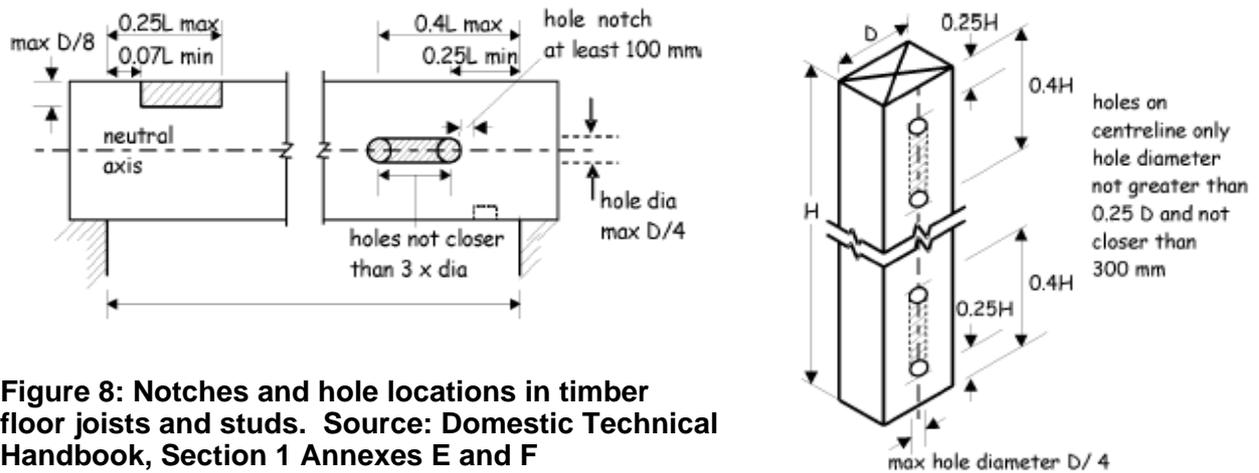
**Figure 8: Notches and hole locations in timber floor joists and studs. Source: Domestic Technical Handbook, Section 1 Annexes E and F**
