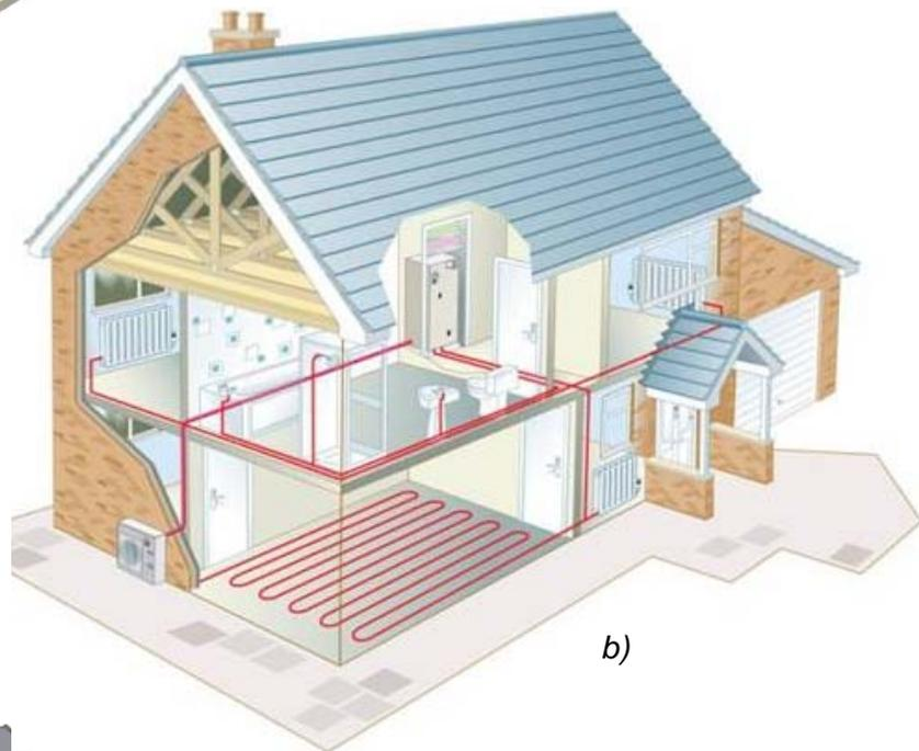
**Figure 2: Examples of air source heat pump Systems.**
