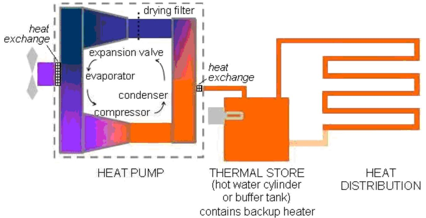
**Figure 1: Schematic of an air source heat pump system**
