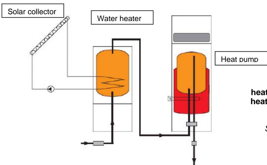
**Figure 4: Solar water heating system supplementing heating by the heat pump, plus integral electric element to provide back up heating**
