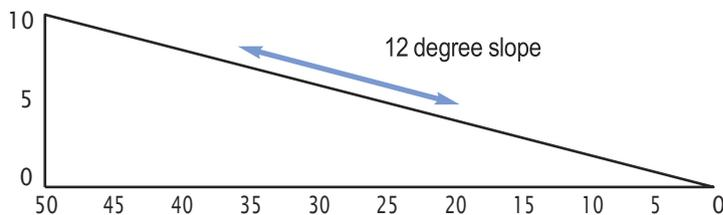
From the diagram above you can see that a 12 degree slope provides a 1 metre rise for every 5 metres travelled on the horizontal plain.
