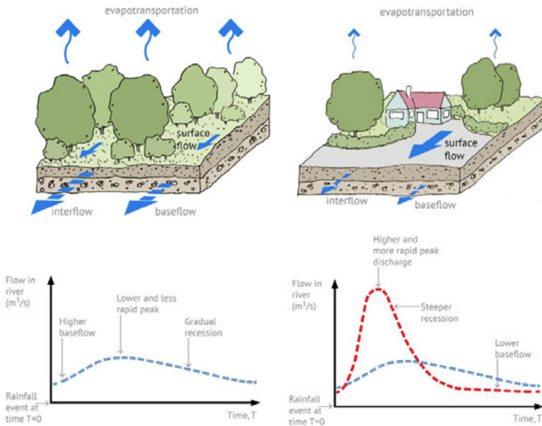
**Figure 4. Overview of surface water flows in a natural catchment and in a developed catchment, illustrating the impact of urbanisation showing increased surface water flows and increased river flows. Illustration courtesy of CIRIA and [www.susdrain.org](http://www.susdrain.org).**
