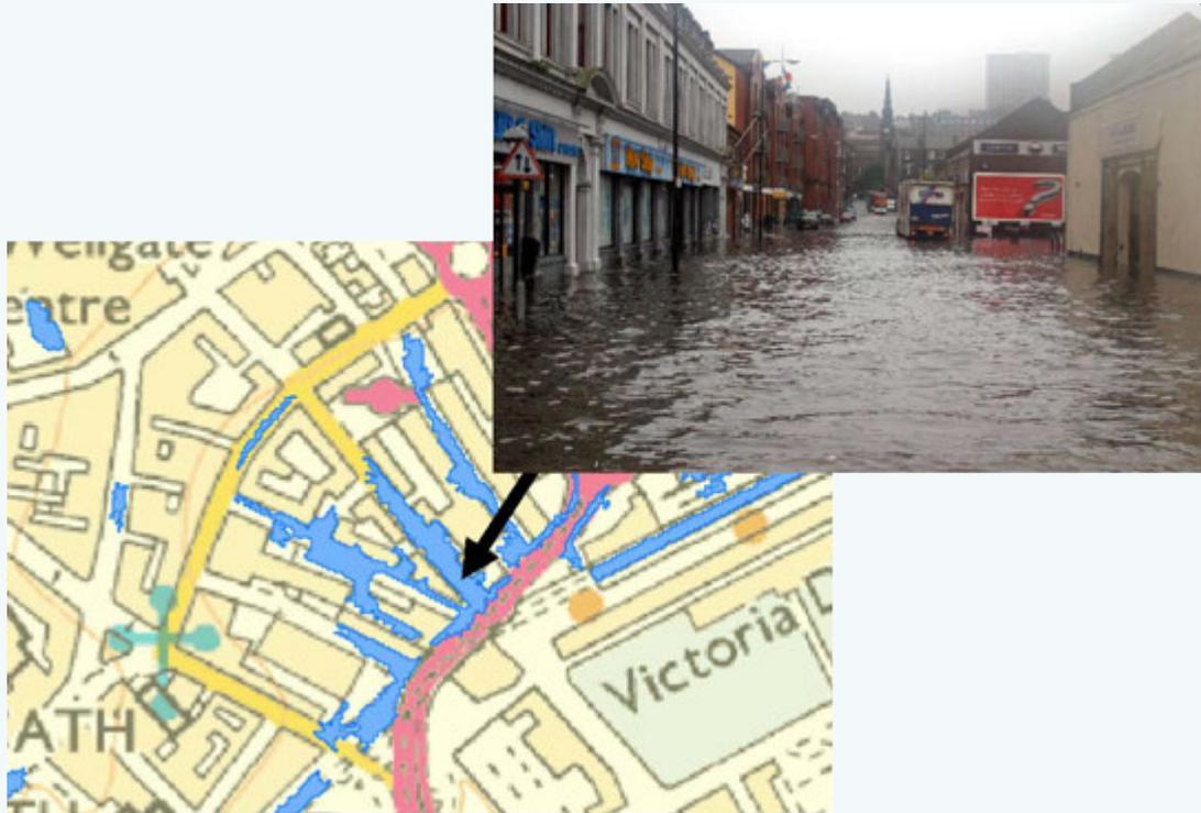
**Figure 9. Comparison of modelled flooded areas and areas of recorded flooding in the Trades Lane area of Dundee. Photograph courtesy of DC Thomson & Co.**
