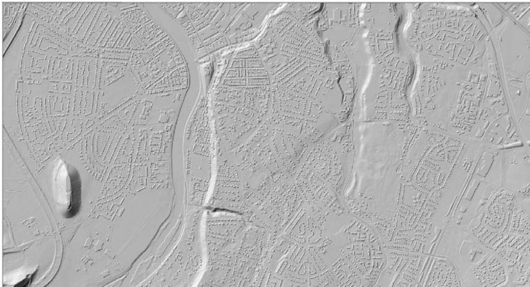
**Figure A1 – Representation of the ground is a key component of surface water flood modelling. The example above is a Digital Terrain Model (DTM) produced from LiDAR data with buildings represented.**
