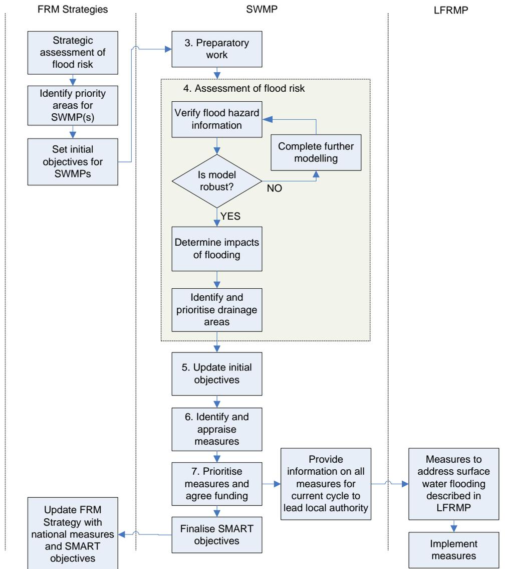
**Figure 6. Overview of the surface water management planning process (numbers in flowchart refer to subsequent sections in guidance).**
