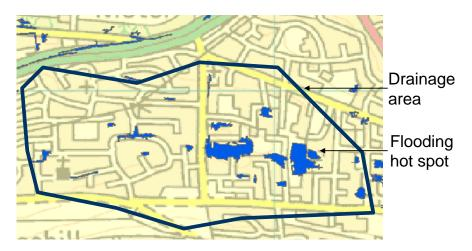
Figure A2 – Indicative example of a surface water flooding 'hot spot' and its associated drainage area.
