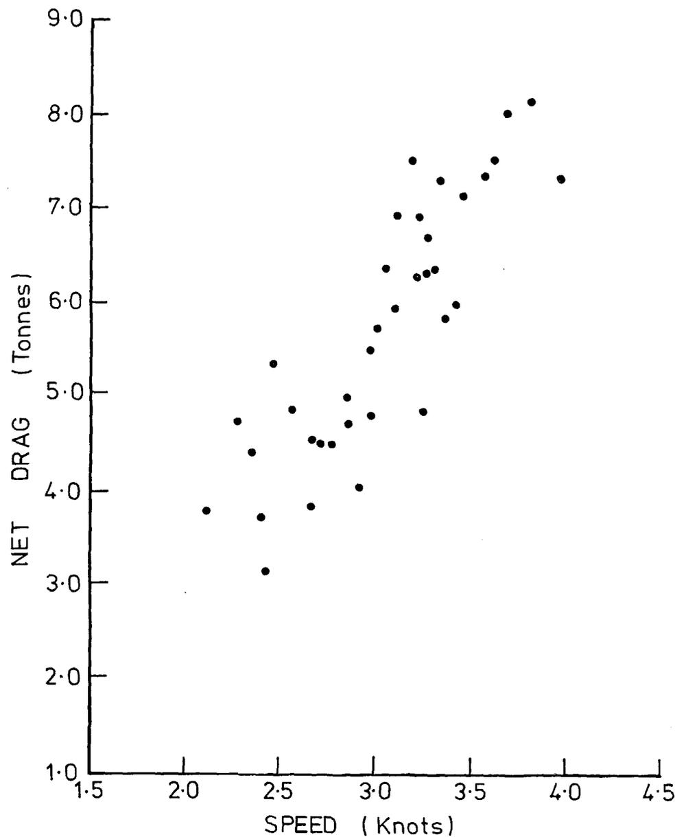
**Figure 3** A typical experimental graph of net drag against speed for a 1000 hp net.
