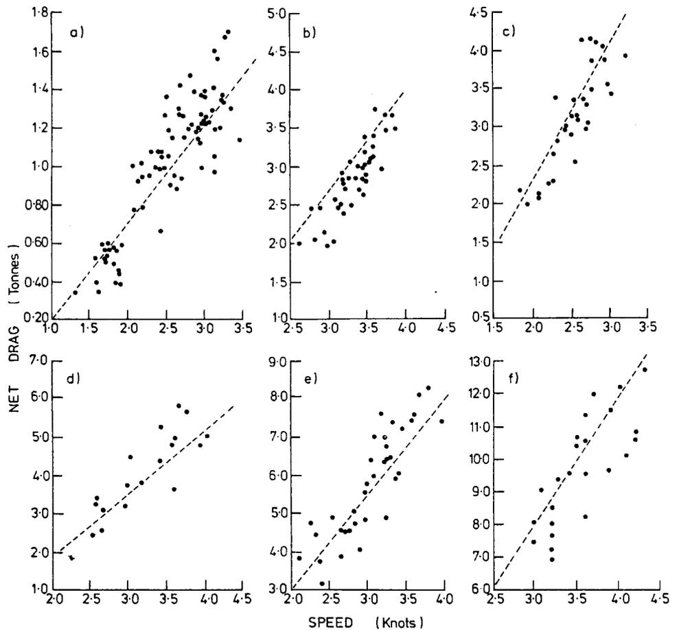
**Figure 5** Comparison of formula predictions with experimental results. Individual points denote the experimental points whilst the dashed curves denote net drag as predicted by equation (8).
