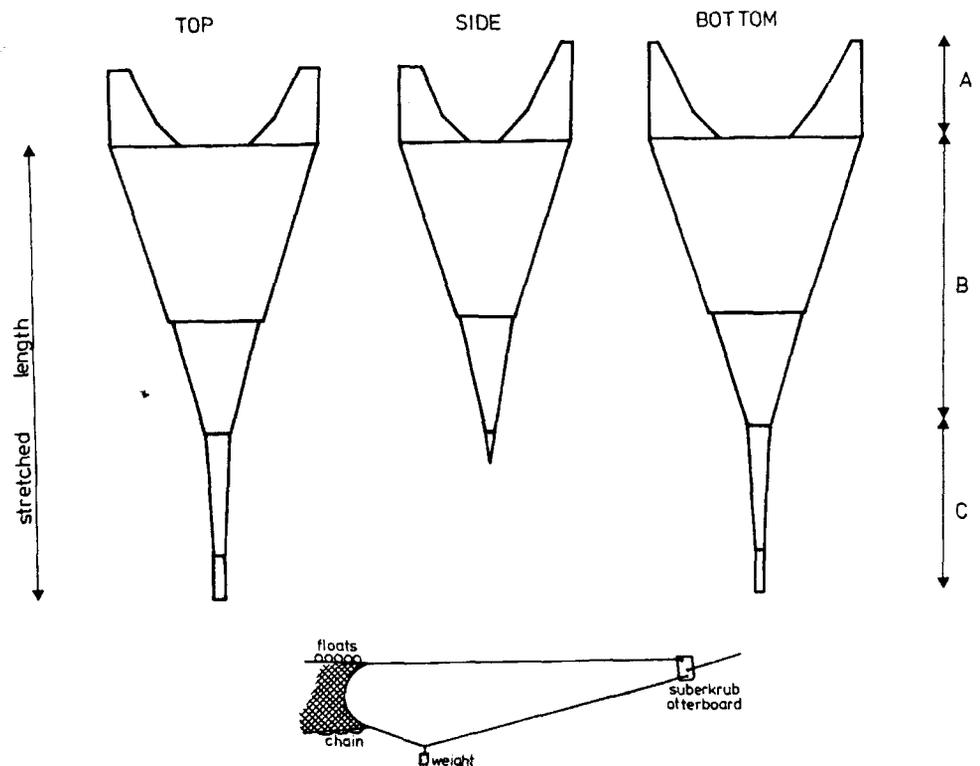
Figure 1 Definition of net sections as in Table I.
