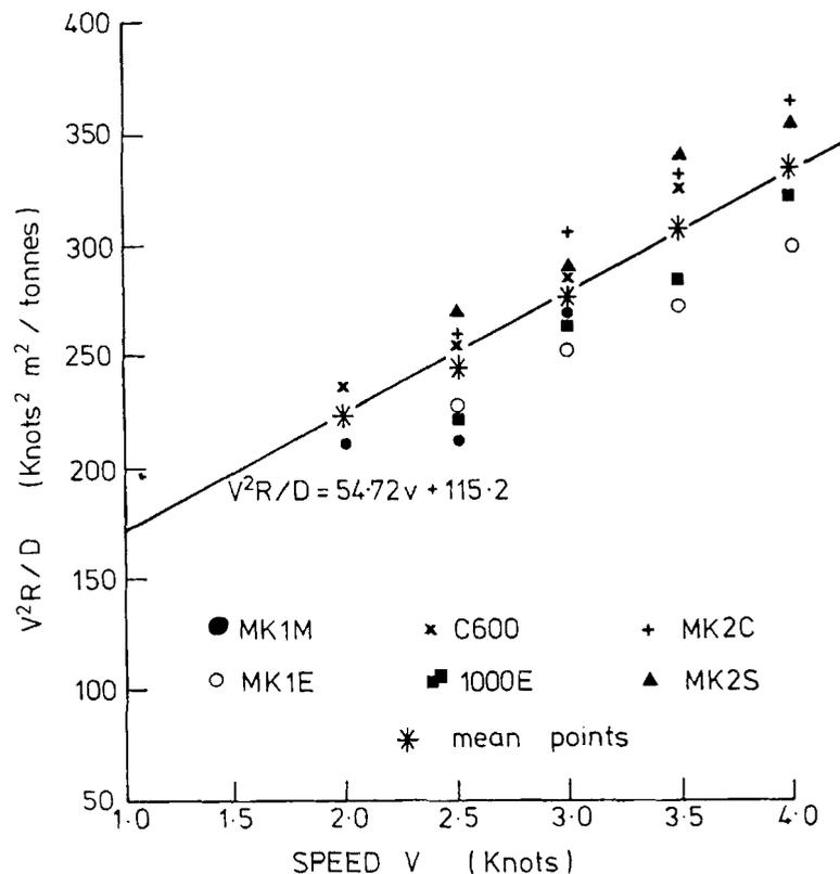
Figure 4 Relationship between  $V^2 R/D$  and  $V$ .
